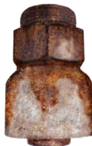
Competitor 2 after 1,000 hours ASTM B117 (ISO 9227) Salt Spray Test
