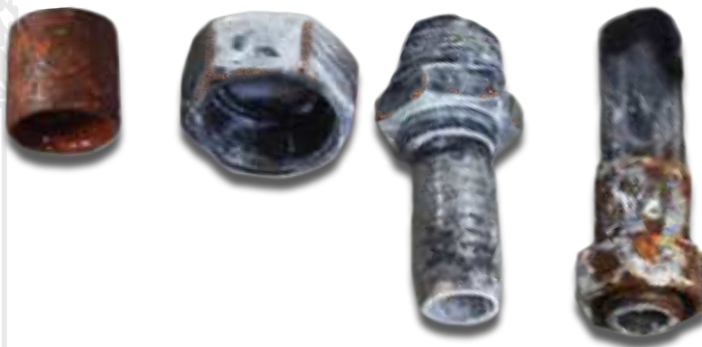
Competitor 1 after 1,000 hours ASTM B117 (ISO 9227) Salt Spray Test
